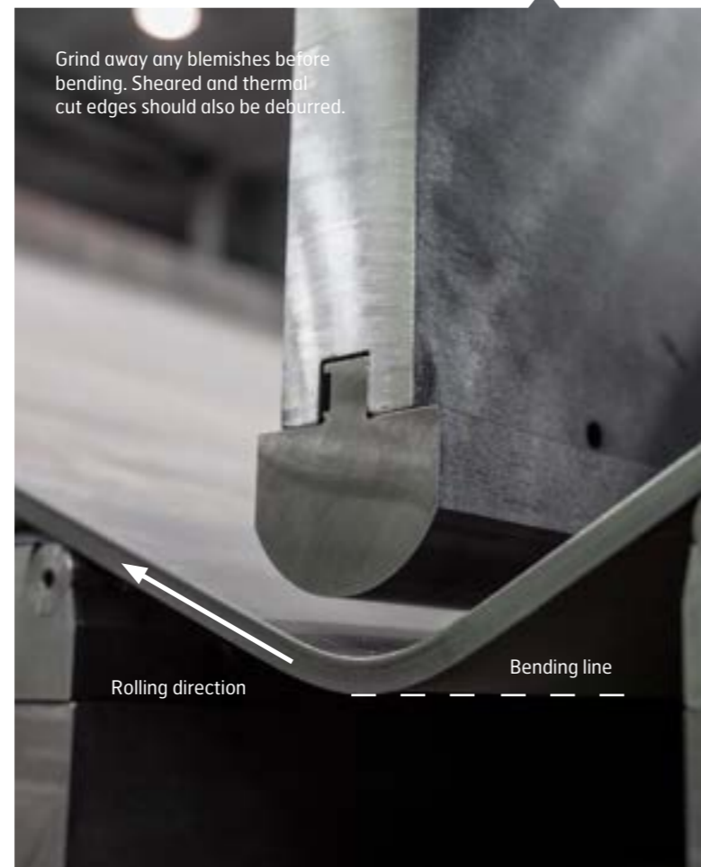
FIGURE 2 Bending transverse to the direction of rolling. The edges of the die opening should always be as hard as, or harder than, the plate being bent, in order to avoid excessive damage to the die. A simple way of achieving this is to mill grooves in the die edges and fit lubricated round rods of, for example, hardened steel into the grooves. The edge radius of the die should be at least half the plate thickness.
