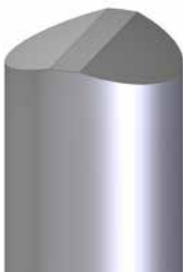
Figure 20. A chamfered punch with a flat centre section.
