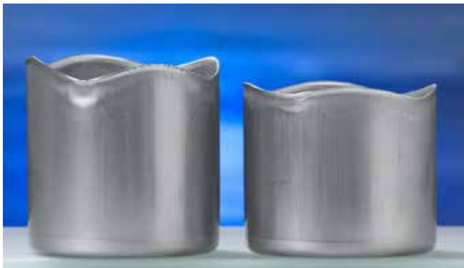
Figure 35. The influence of lubricant viscosity on drawing. Maximum cup height using lubricant viscosity 500 cSt (left cup) and 40 cSt (right cup).
