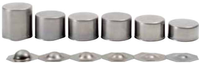
Figure 5. Maximum cup height and dome height for deep drawing and stretch forming, respectively. Steel grades (from left to right): CR5, Docol 600DP, Docol 800DP, Docol 1000DP, Docol 1200M and Docol 1400M.
