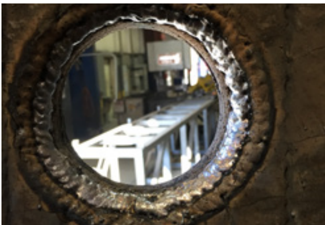
Opening in a Duroxite® plate hardfaced with Duroxite® AP WIRE to protect the part without needing to move the assembly.
