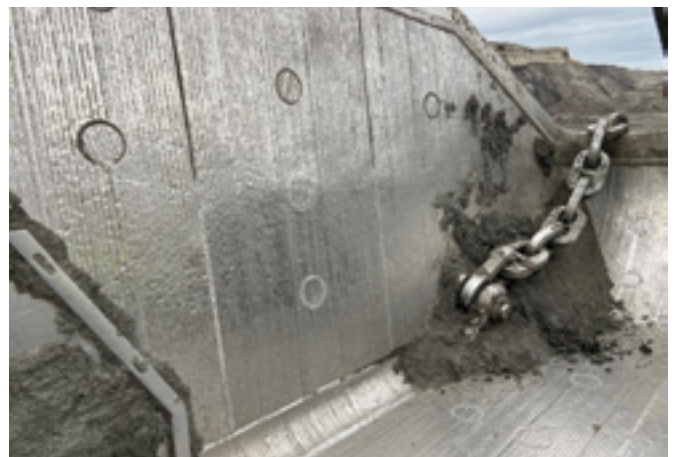
Plug welds with Duroxite® WIRE to protect the soft joining wire that is used to secure the Duroxite® plates.
