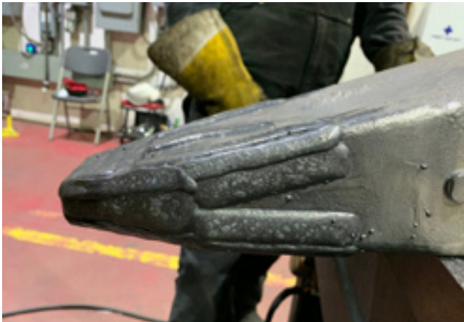
Ground engaging tool (GET) hardfaced with Duroxite® 200 WIRE.
