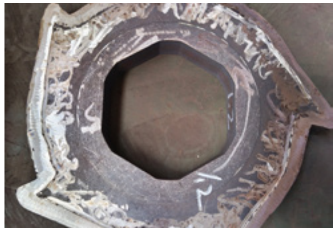
Shredder rotor hardfaced with Duroxite® AP WIRE.
