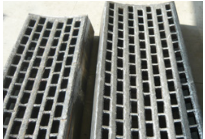
The insides of screen holes protected with Duroxite® 100 WIRE.
