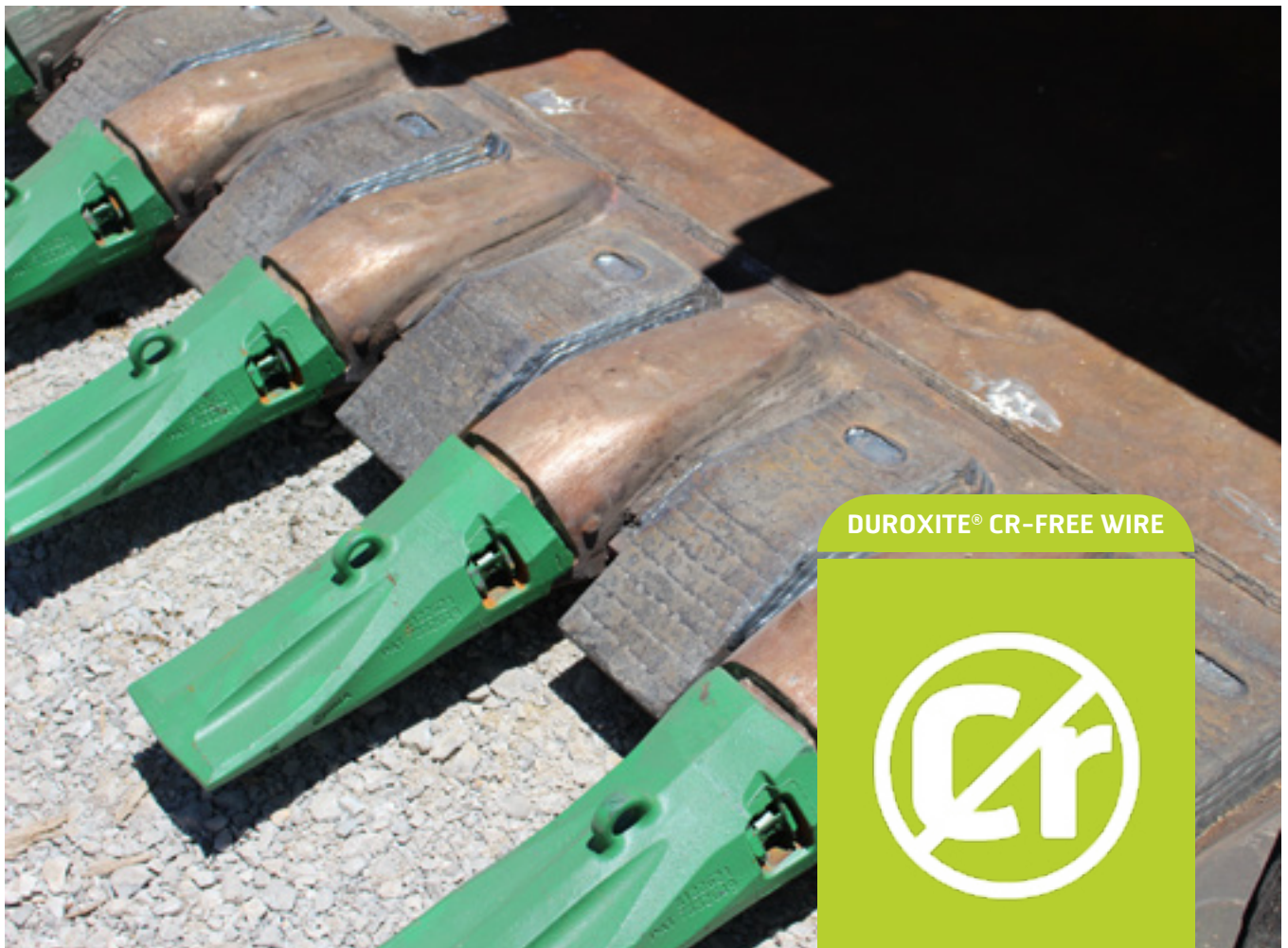
Lip shrouds welded with Duroxite® Cr-Free WIRE.
