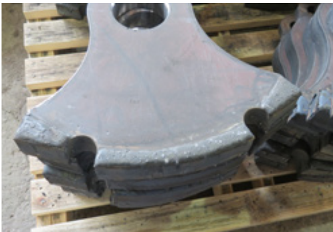
Recycling hammer hardfaced with Duroxite® 300 WIRE.
