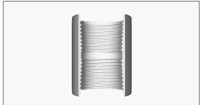
Figure 6. Splice sleeve of RDT piles
